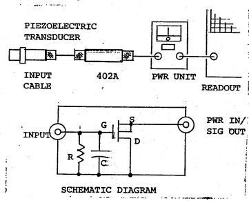
Figure 2 Typical Application Series 402A
