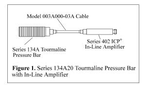
The Tourmaline Pressure Bars is a high-pressure, fast rise time, suppressed-resonance blast sensor ideal for single-shot, high-frequency measurements of incident or reflected shock wave pressures found in studies of plasma physics and hyper-sonics. Ranges up to 20,000 psi are available.
